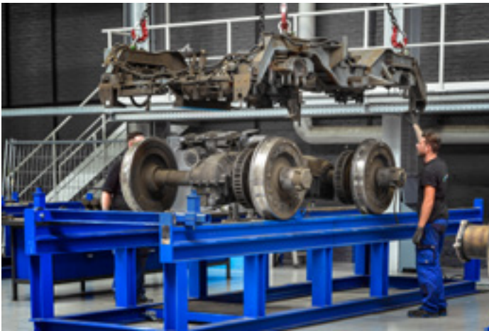
Maintenance des bogies
